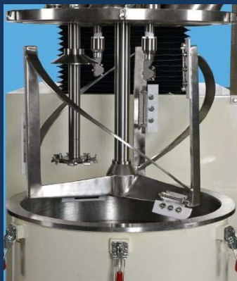
Dual-Shaft Mixer composed of a three-wing anchor with helical flights and scrapers, and a saw-tooth disperser with slinger. Two clean-in-place rotary spray nozzles are also shown.
