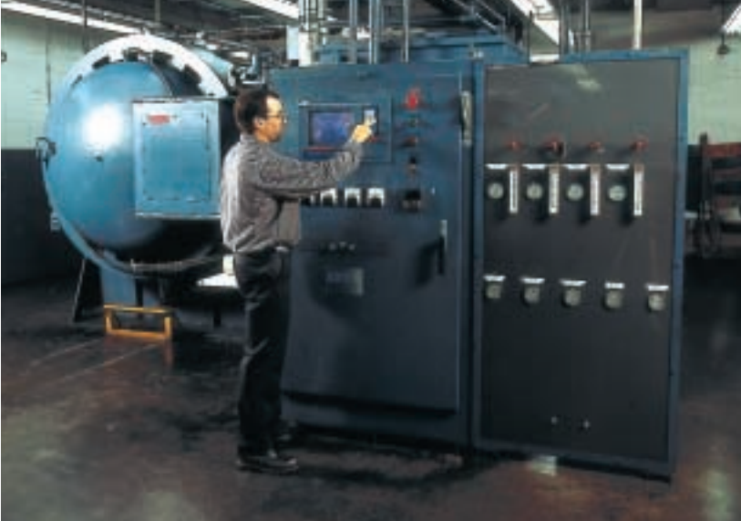
Using the sinter hip process, Vista offers a product that is 100% free of microscopic voids.
