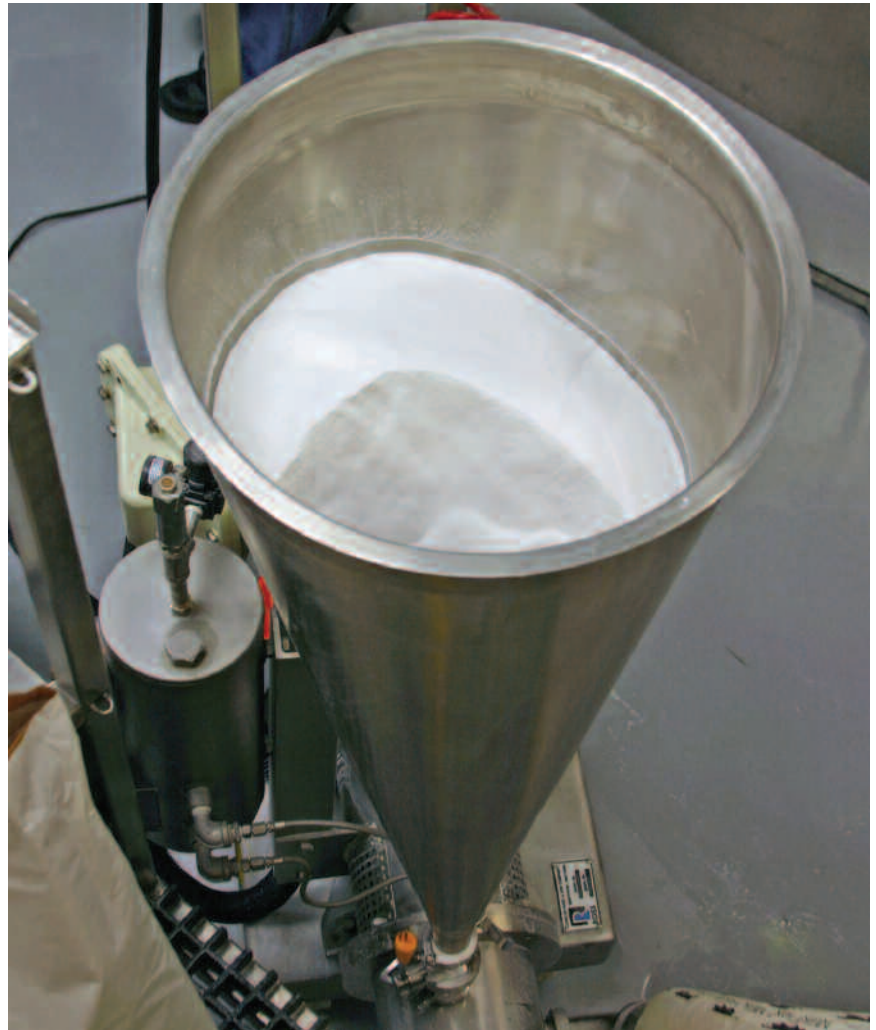
Solids in the mixer's overhead hopper are drawn under vacuum directly into the high shear chamber, where they are instantly dispersed into the liquid stream. Photos courtesy of Botanical Laboratories.
