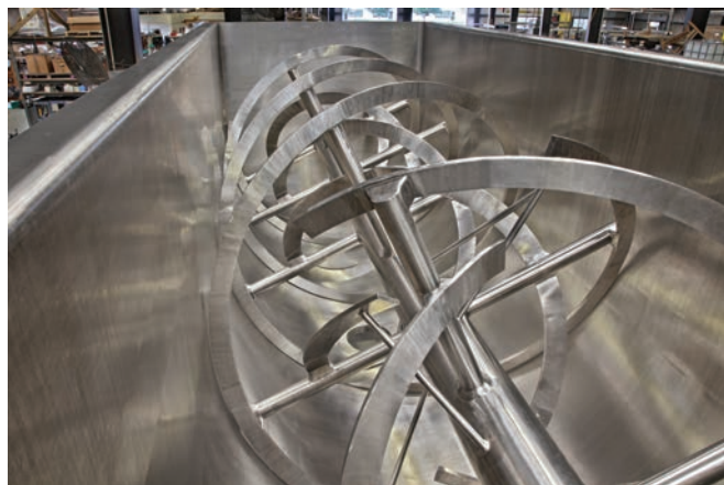
Figure 1. A typical ribbon blender agitator consisting inner and outer helical ribbons supported by spokes welded to a solid steel shaft.
