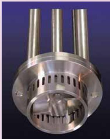
Figure 1 – Rotor/stator assembly of a batch high shear mixer.
