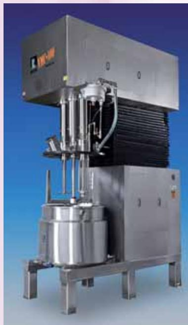
Figure 2 – Multi-shaft mixer equipped with three independently-driven agitators: a high speed disperser, a rotor/stator mixer and three-wing anchor agitator.
