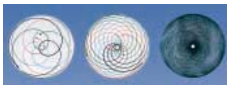
Left: blade motion during 1 revolution. Center: 3 revolutions. Right: After only 36 revolutions, the blades of the mixer have contacted virtually the entire batch.
