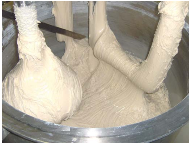
Highly filled potting compound batched in a planetary disperser.
