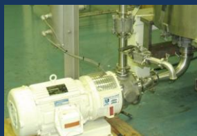
Explosion-proof high efficiency motor. Stainless steel and/or washdown duty motors available.
