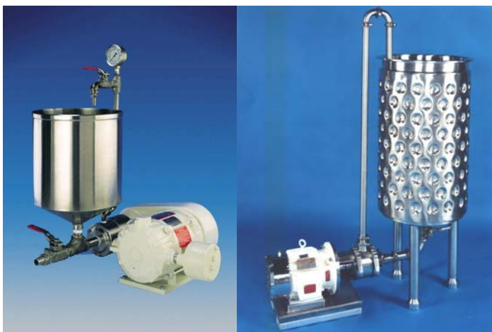
Single-stage inline high shear mixers are available in laboratory (left) and production (right) models up to 100HP. At relatively low viscosities and volumes, the recirculation vessel does not normally require any additional batch agitation.
